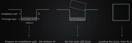
Prepare an installation well, the bottom of the well should be with sand or soil to help drain.
